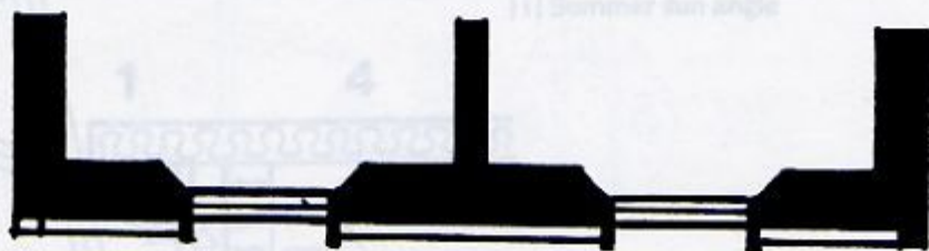
COMBINATION OF TROMBE WALL AND DIRECT GAIN WINDOW.
