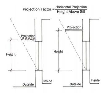
Note: Overhangs located directly above the window head need the least projection.
