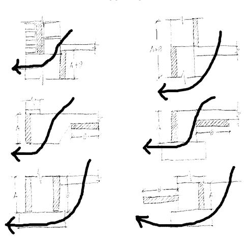
The following slab insulation installation details meet the intent of the code.
