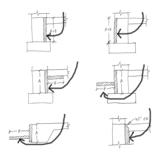
Drawings in this manual are intended only to show placement of insulation, and are not to be used for structural design, moisture protection design, or other uses.
